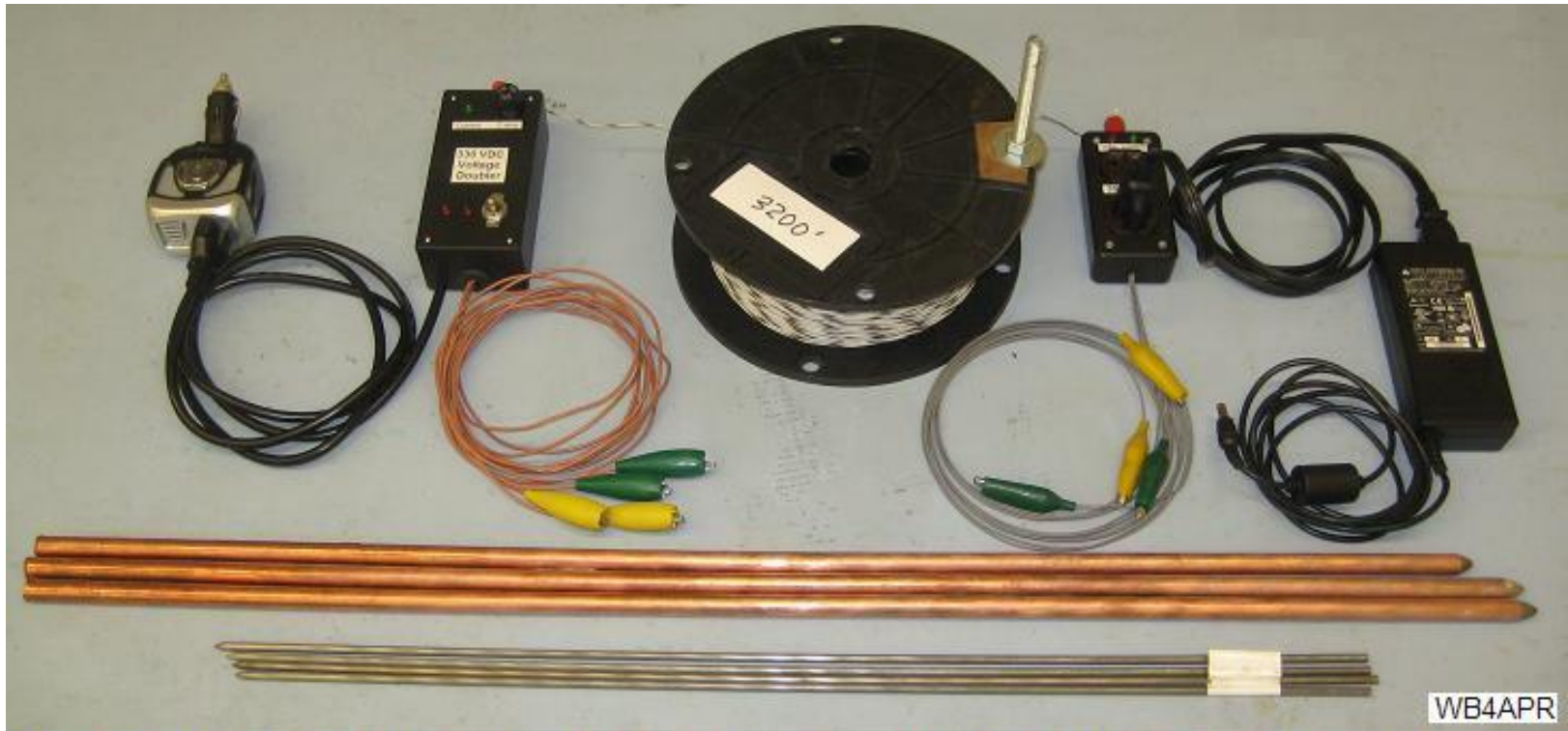
Left to right: 12v Inverter to 115 VAC, Doubler to 330 VDC, 3200' wire, Outlet box, Laptop Power Supply 18v at 4.5 amps.
